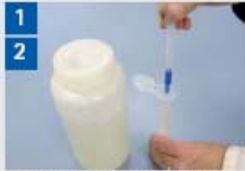
1 2 - Collect fuel sample (1 litre) - Collect blue Capture Solution from sample tube w small pipette
